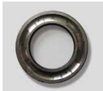
Klüberplex BEM 41-141 attained maximum run-time of 50 hours.
