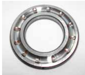
Competitor product 2: wear limits were exceeded so test had to be stopped after 39.6 hours.
