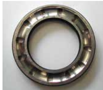
Competitor product 1: wear limits were exceeded so test had to be stopped after 13.5 hours.
