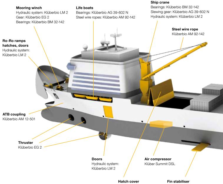
This illustration shows the various applications of our marine lubricants. To show as many applications as possible in one illustration, we included components of the following ship types in this synthetic ship: Ferry, cruise ship, cargo ship, wind turbine installation vessel, anchor handling tug supply vessel.
