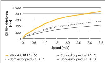
Klüberbio RM 2-100 achieves higher oil film thickness in hydrodynamic operation than other EAL stern tube oils.
