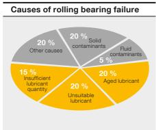
55 % of rolling bearing failures could be prevented through the use of Klübermatic lubricating systems!
