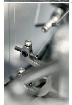
Hosiery knitting machines (stitch-forming elements, gears and bearings)
