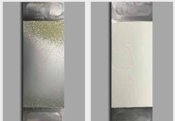
Standard EP2 grease after test: 88 % spray-off
