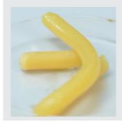
Klüberplex HB 98-601 BH sample before starting the test
