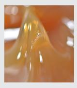
Klüberplex HB 98-601 sample after testing at more than 200 °C for 3 hours
